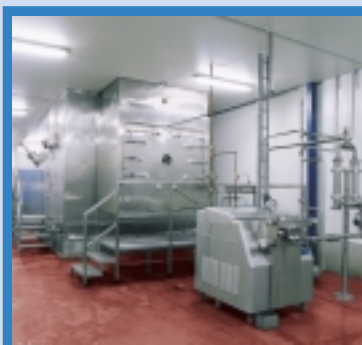
Model NC-10 spray dryer in Angers, France evaporates 3,000 lb/hr water and produces high quality product.
